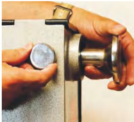
▲ You lock the pulley wheel by pulling out and rotating this disc
